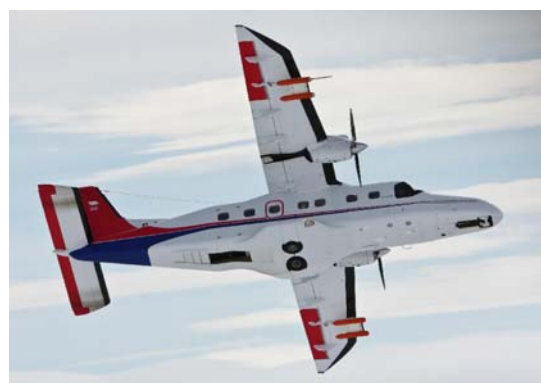
Figure 1 Dornier 228 showing instrument bays for ground viewing sensors.
